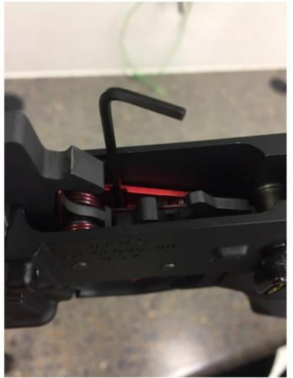
When installing your Timney Calvin Elite AR-15 trigger be sure to tighten down the set screws once the pins and safety are in place. No torque wrench is necessary, hand tightening should be sufficient.
