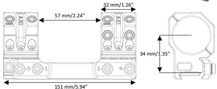
The mounts are machined from billet 7000 series aluminum and all aluminum parts are hardcoat anodized. The Torx 20 ring screws are zinc-nickel coated for corrosion resistance and come pre-waxed from the factory to ensure proper torque values. The levers can be adjusted for tension.
